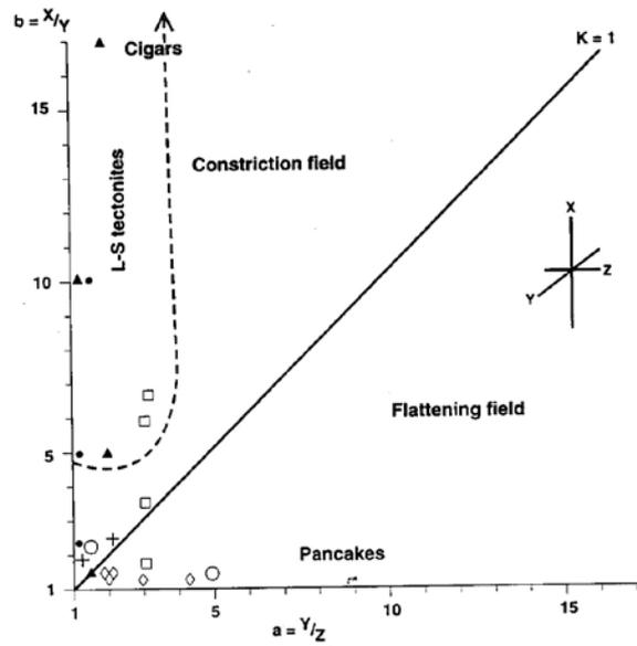
**Flinn diagram displaying strain states in conglomerate**
