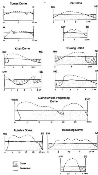
**Figure 2:** Cross-sections of basement domes shown on Fig. 1. Tumas Dome section from Jacob *et al.* (1983); Namibfontein-Vergenoeg section from Kröner (1984); other sections drawn from Smith (1965) and from the author's field mapping.
