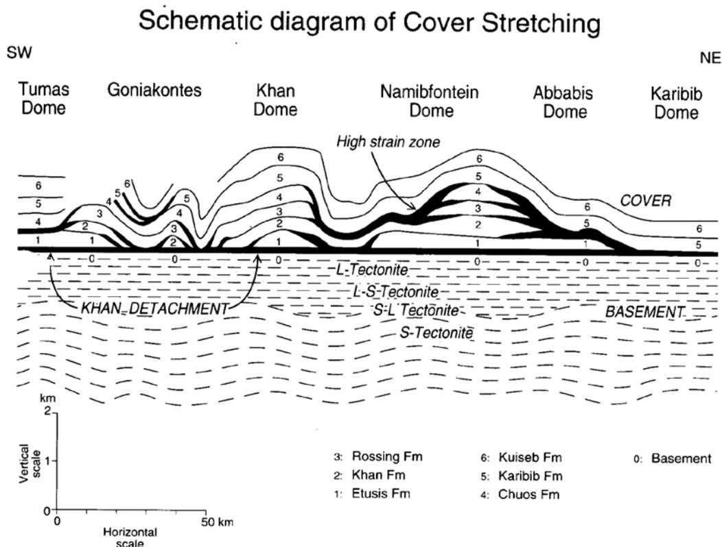
**Figure 5:** Cartoon of how the cover has been stretched out over the basement following detachment and doming. To simplify the cartoon, the effects of doming have been removed so that the Khan River Detachment is now horizontal. Formation names and distribution of formations taken from Smith (1965). Line of section AA' given on Fig. 1. Note the great vertical exaggeration.
